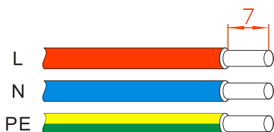
Figure3-21 Stripping diagram of AC output (unit: mm)
