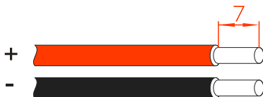
Figure3-16 Stripping diagram of DC input (unit: mm)
