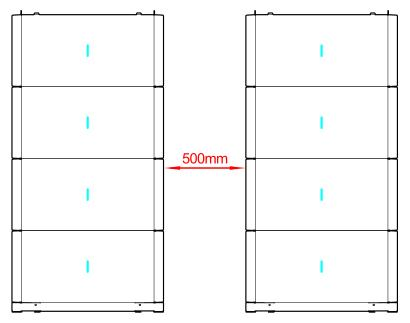
Figure 3-21 Distance between the batteries
