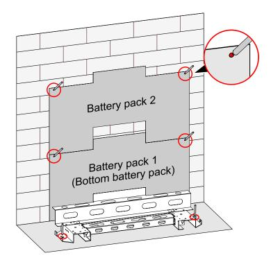
Figure 3-8 Mark the installation holes
