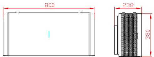
Figure2-4 Battery size (Unit: mm)
