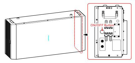
Figure3-25 Battery ON/OFF button position
