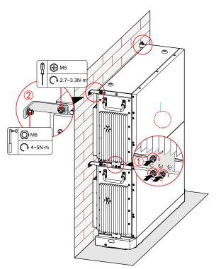
Figure 3-20 Tighten the top battery pack
