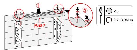
Figure 3-16 Assemble the support and base
