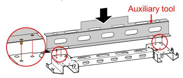
Figure3-5 Install auxiliary tool
