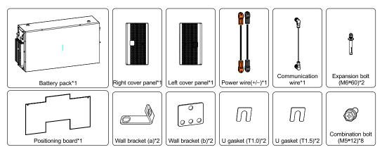
Figure 3-4 Battery pack packing list
