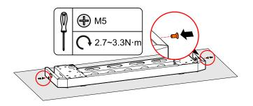
Figure 3-11 Fasten the cover plate
