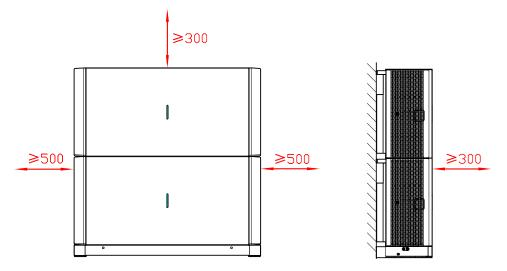
Figure 3-3 Installation space (unit: mm)
