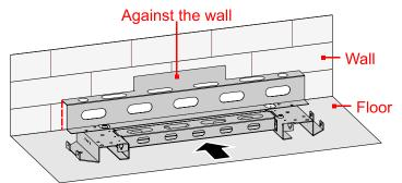
Figure3-6 Auxiliary tool against the wall
