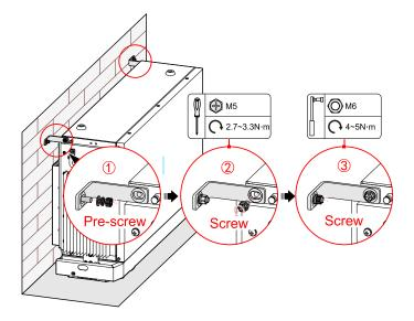
Figure3-18 Fix the wall bracket a
