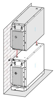
Figure 3-19 Place the battery pack
