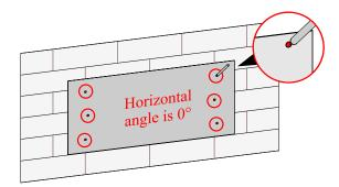
Figure 3-13 Mark the installation holes
