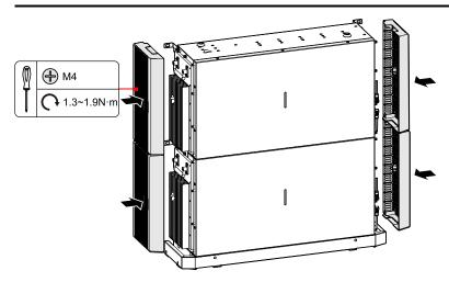
Figure 3-24 Tighten the wiring cover plate
