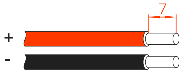
Figure3-36 Stripping diagram of DC input (unit: mm)
