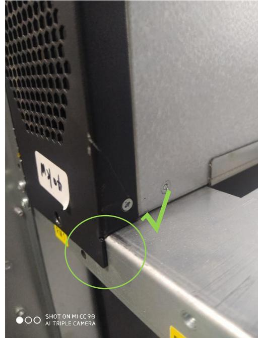
From the interface side of charging module to check if correct installed, as pictures show below.
